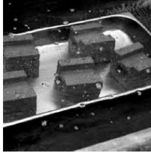
Fig. 2 Water Absorption Test
